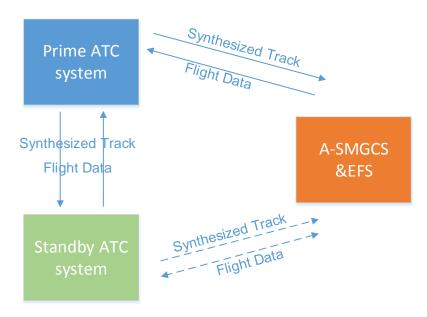
These systems together supports fight handover via screen, go-around info and departure flight sort and display. Also switchover of prime and standby systems have no effect to other systems.
