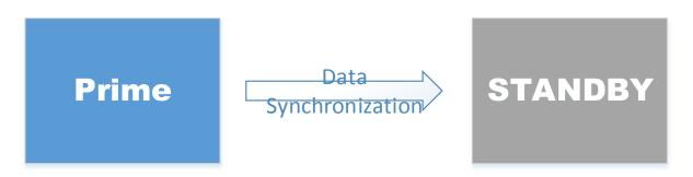
The ATC system supports prime and standby mode. Data is only transmitted from the prime system to the standby system. The transmitted data includes synthesized track, flight data, and control operations, to make sure data in the standby system is the same with in active system.
